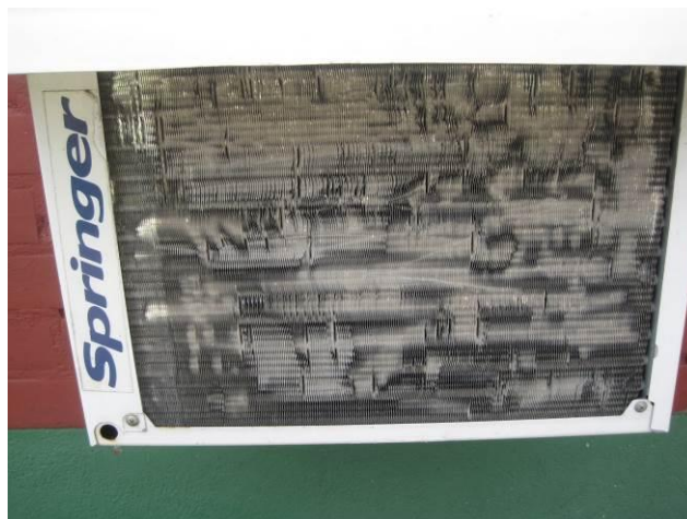
Figure 31: Major Deformities in Heat Exchanger Ribs
